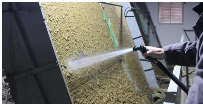
Manure washed from the dairy runs over a separator screen that allows liquid to drain away. The liquid is treated for other uses on the dairy while solids are incorporated as crop fertilizers.
