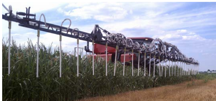
The VanTilburgs fashioned a cover crop seed planter from a highboy sprayer.
